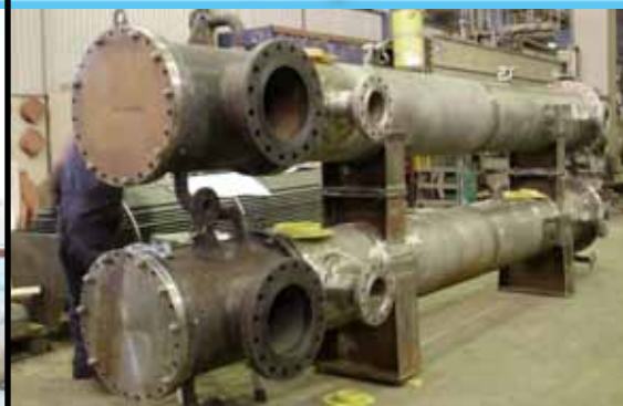
Crude Heat Exchanger for Draugen
