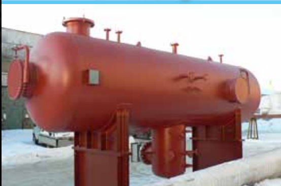
HP Flare Knock-out Drum for Ormen Lange
